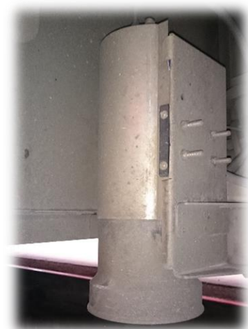
Figure 2: Field installation with additional stone protector
